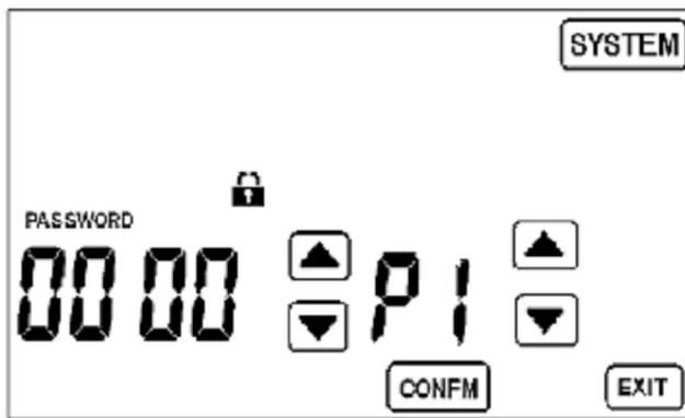
Press or on the left to change the password. P1 indicates that the 1st digit password (read from left) is selected. Press or on the right to select the digit. After setting all 4 digits, press CONFM to activate the security mode.
