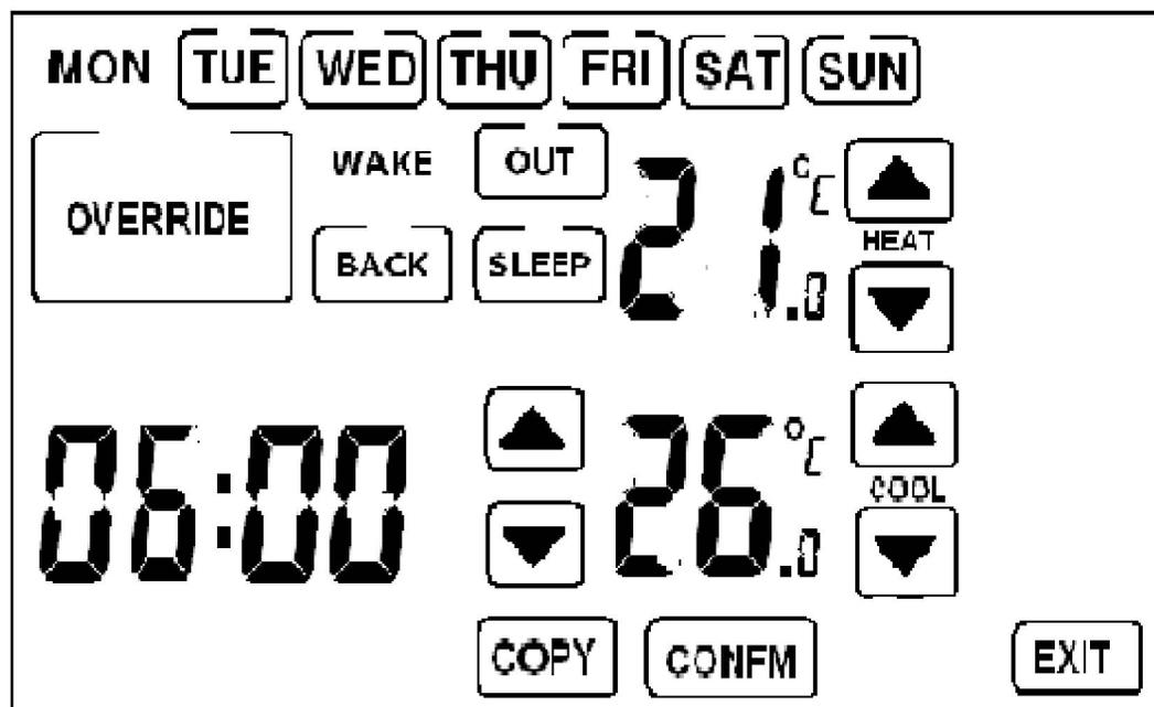
4. Press DOWN / UP to change the time, heat and cool setting temperature.
